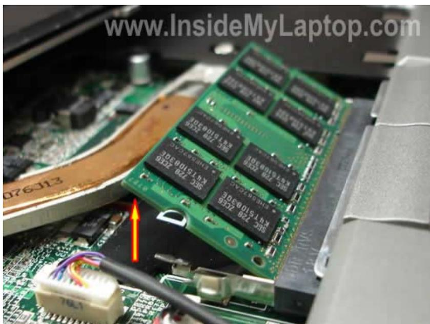
Pull the memory module from the slot A by the edges.
